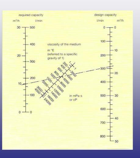
The capacity specified in the pump performance charts generally refer to water (1 mPas).
