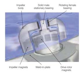
The patented impeller of Alfa Laval magnetic mixers levitates on a magnetic field, which greatly reduces friction and maximizes cleanability.
