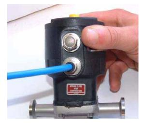
**2.** Remove the fasteners and the valve actuator.
