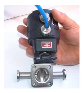
**5.** Remove diaphragm from actuator by turning anti-clockwise.
