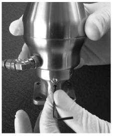
18. Once the spindle adaptor locking screw is undone, remove the spindle adaptor and compressor assembly from actuator bonnet.
