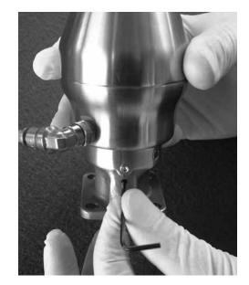
22. Gradually tighten rotation grub screw until actuator bonnet is secure using table two below.
