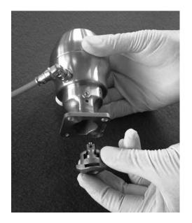
20. Apply Loctite 222 to spindle adaptor locking screw. Insert spindle adaptor and new compressor assembly into actuator bonnet until fully located.
