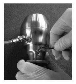
16. Rotate actuator bonnet until breather hole lines up with the spindle adaptor locking screw.
