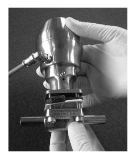
3. Inspect the valve body sealing surfaces for damage.
