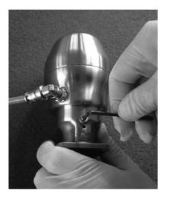
23. Re-attach the actuator to the valve body. Repeat steps 6 to 14.
