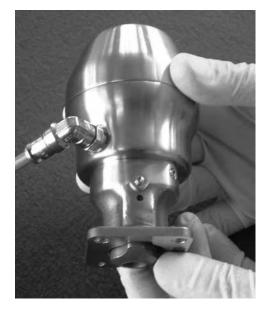
21. Insert Allen Key into actuator bonnet hole and tighten spindle adaptor locking screw fully using table one below.
