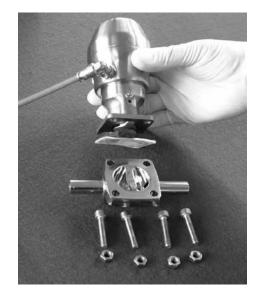
5. Remove diaphragm from actuator by turning through 90° (PTFE Diaphragm). For rubber diaphragm unscrew in anti-clockwise direction.
