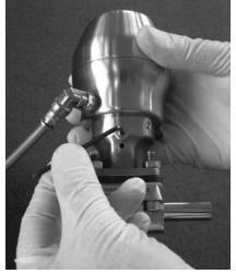
25. Rotate actuator cylinder while actuator is attached to the body, until inlet port is in the required orientation. Rotation feature available on sizes DN15 (0.5 in.) - DN50 (2.00 in.). To facilitate rotation please ensure air supply is "on" for spring closing mode and "off" for spring opening mode.
