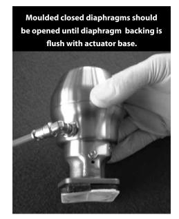
7. For PTFE diaphragm please engage diaphragm bayonet into the compressor slot by applying pressure to the center of the diaphragm. Ensure correct engagement. Continue to apply pressure to the center of the diaphragm and turn through 90°. For rubber diaphragm screw in clockwise direction and avoid over-tightening
