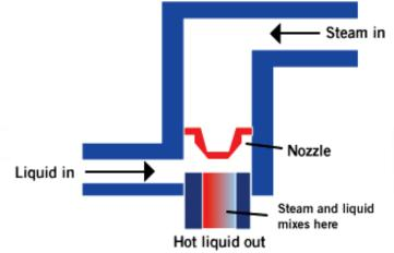
Image  ${\bf 1}$  - In direct-contact steam heating, steam is injected directly into the liquid
