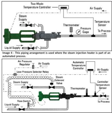
Image 5 - In this configuration, the steam solenoid valve automatically stops steam flow when the liquid flow stops.
