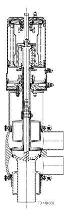
Fig. 1 Details of Unique PMO-F Mixproof Valve
