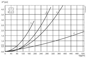
Fig. 4. Pressure drop/capacity diagram, lower body.
